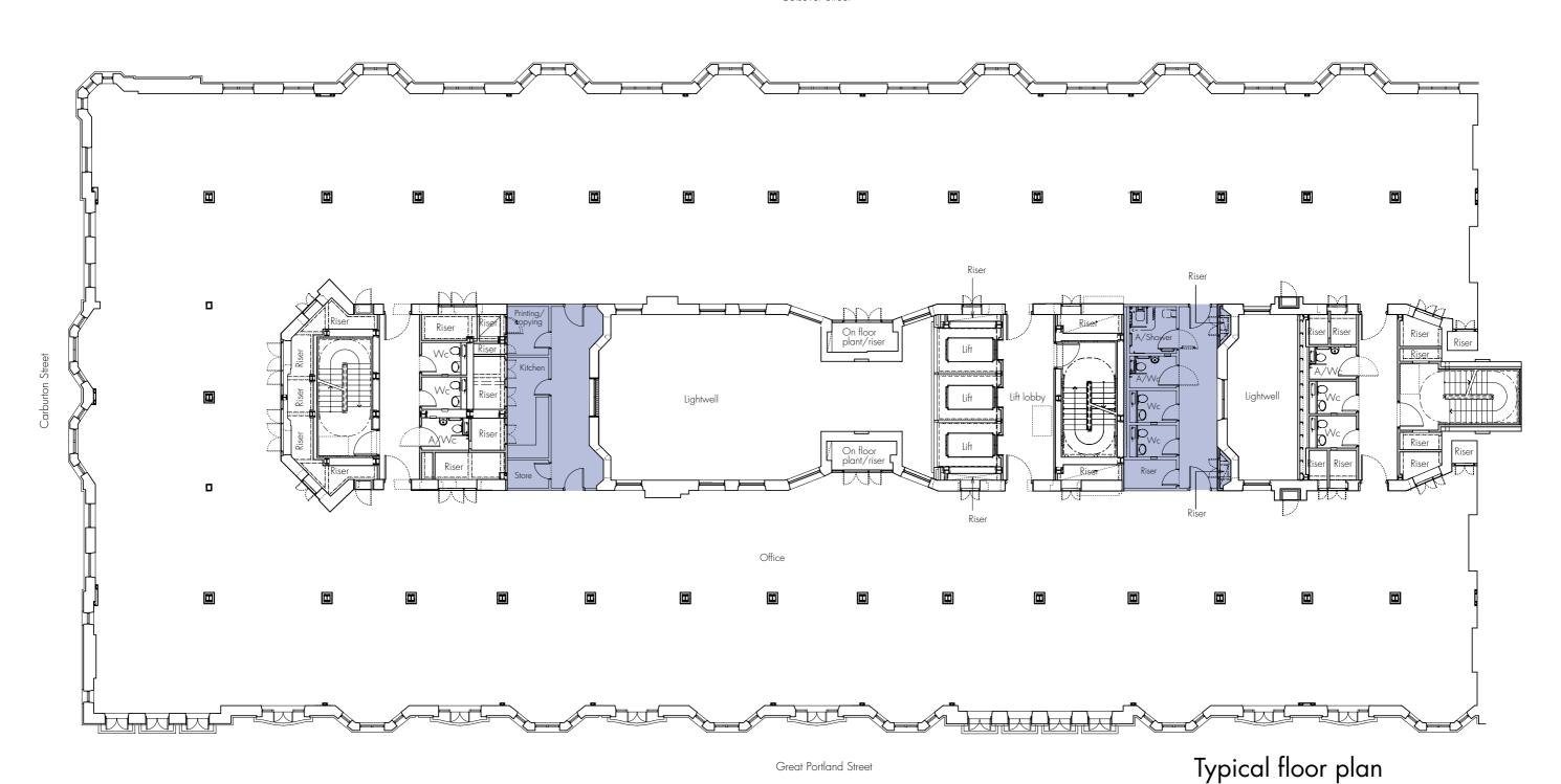
Core 1 - Location of kitchen is readily serviceable via capped connections installed as part of the base build scheme, i.e. drain, SVP, and cold water supply
